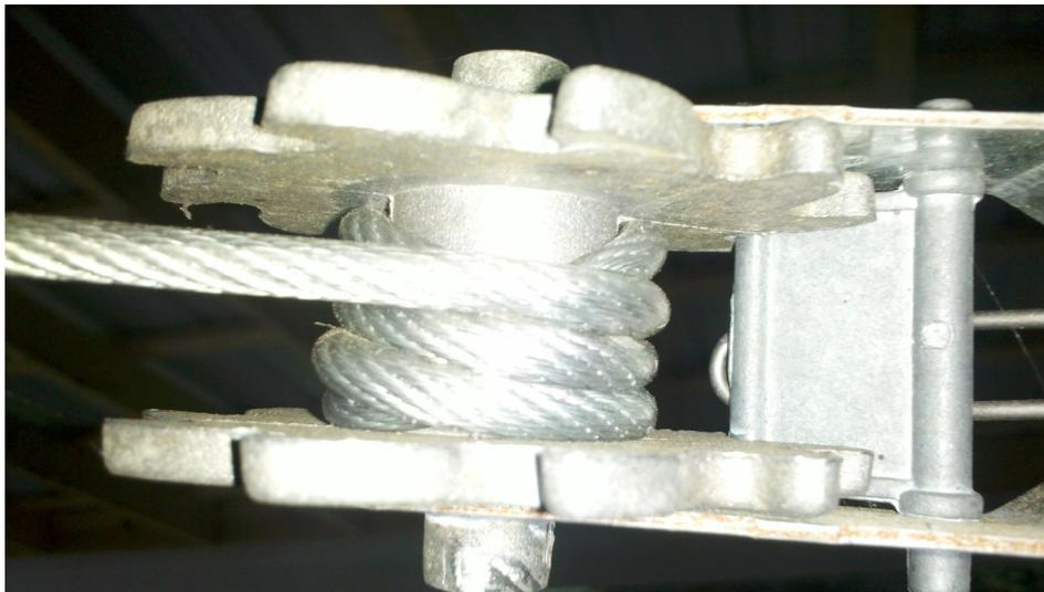
**The Cable Tightener has a drum with holes in it. Just push the Cable end through the holes—pull out—leaving a tail. Wrap around more Cable over top of the tail.**
