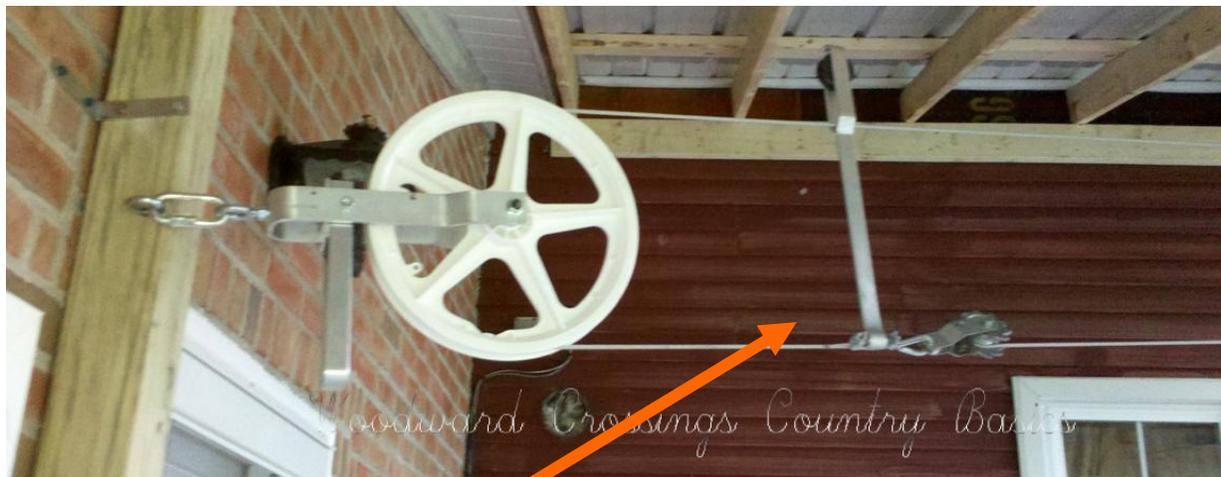
**Use the Inline Spacer and Cable Tightener at the beginning.**
