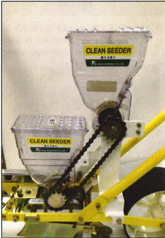
6. a. Place drive chain on both sprockets. b. Pull back on Bracket B until chain is tight. Tighten Bracket B to Bracket A.
