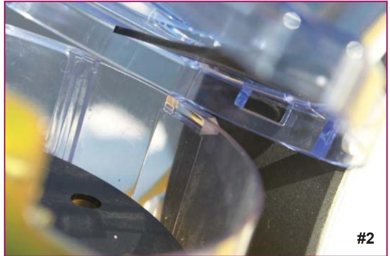
3. Remove the hopper by pushing the two black release clips down on back of hopper. (Photo 1) Slide the hopper forward to release the hopper from the front plastic tab. Be very careful when doing this or you can force the hopper up causing a break in the slot in front of the hopper. (See Photo 2)
