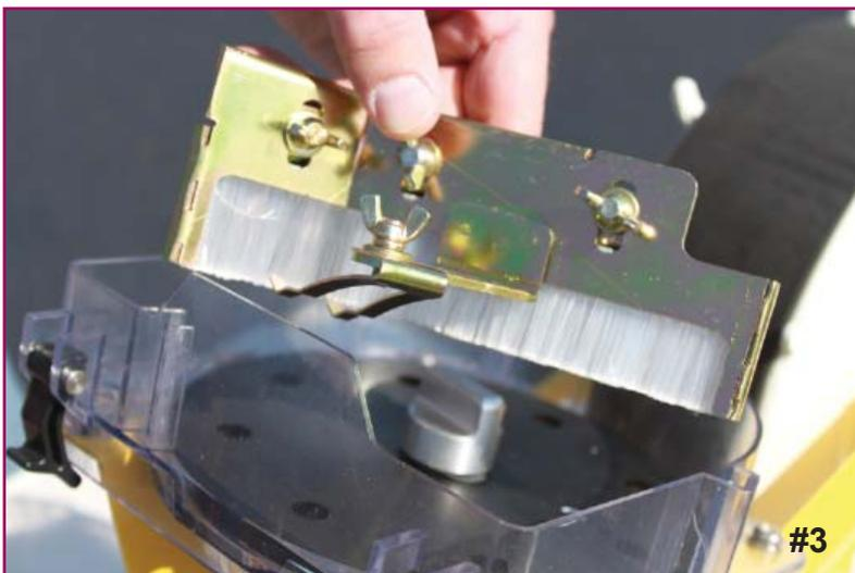
4. Remove the brush assembly by just lifting it up and out. The brushes can be adjusted up or down by loosening the wing nuts. (Photo 3)
