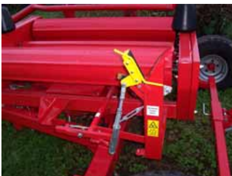
Simple and effective mechanical cut'n hold requires no separate action from the operator.
