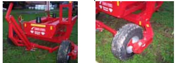
The right side wheel swivels out for more stability when wrapping, swings in for narrow transport.
