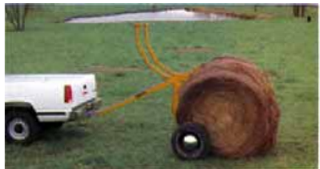
2 Continue backing until loading arm falls over frame of cradle and touches hay
