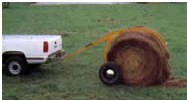
3 Pull forward slowly and the bale rolls on the cradle
