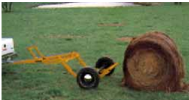
1 Back up to a bale, engage brake switch
